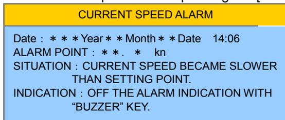
**Fig. 4.1.3 Ex.: Current speed alarm**
