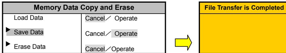
④ When the memory preservation data of SSD is normally copied onto the USB external memory, the message of "File transfer is completed" is displayed on the display screen. (\*6)
