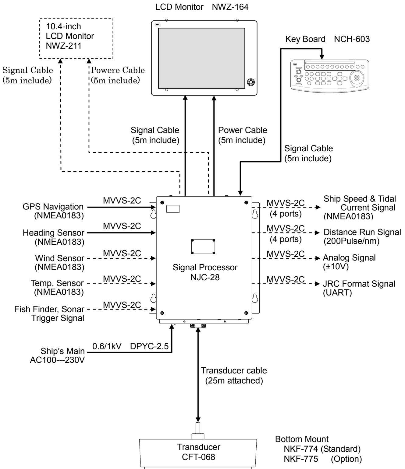
Fig. 1.5-1 JLN-650 Doppler Current Meter System Configuration
