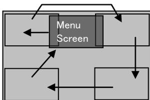
It moves to the table and the graph where it wants to set "Selection frame" with the right and left cursor key. Under such a condition, when the [MENU] key is pushed, a set menu corresponding to the part selected by "Selection frame" is displayed.
