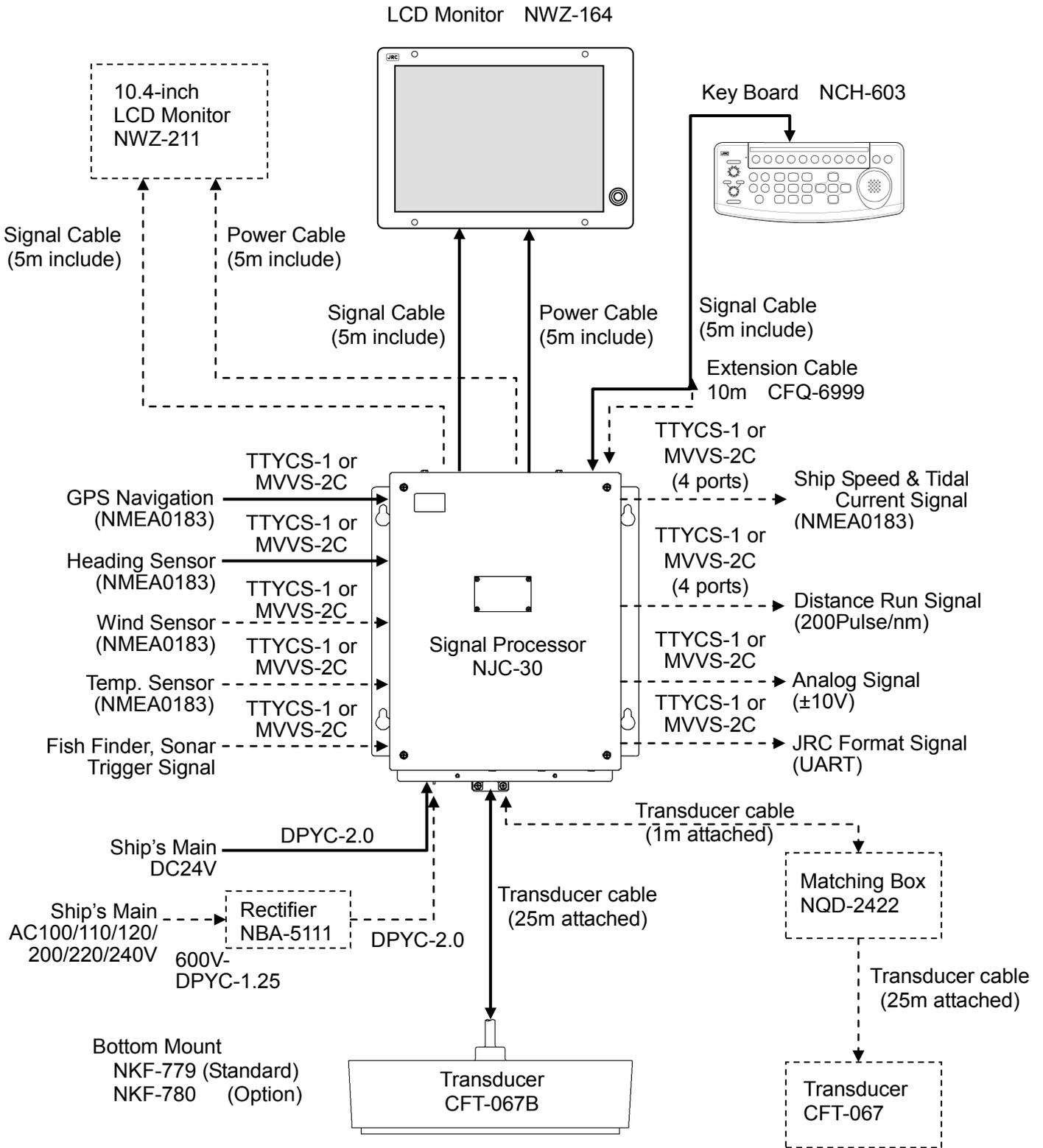
**Fig. 1.5-2 JLN-652 Doppler Current Meter System Configuration**
