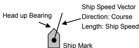
**Operation** **Standard Menu:** Plot screen setting menu/Ship speed vector length: 4 cm/10kn
