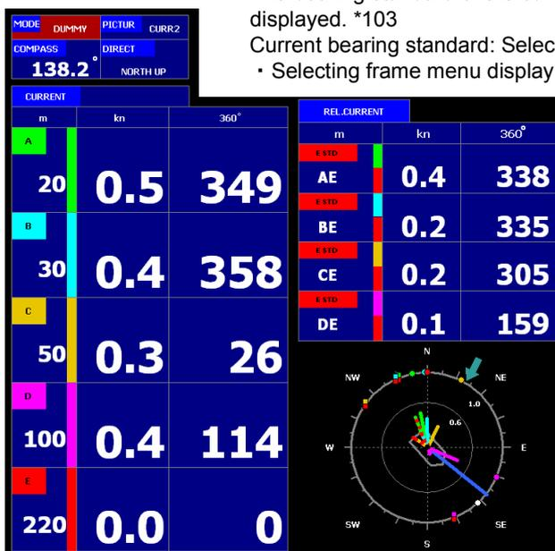
**Relative Current: Current Direction/Speed and Standard Layer:**
