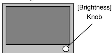
The whole of the screen lightens if the [brightness] knob is turned clockwise.
