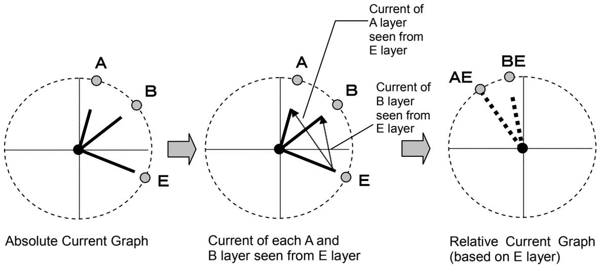
Fig. 6.1.3 Example of Absolute Current and Relative Current Graph Display
