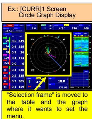
"Selection frame" (outside frame with square yellow bold line) is displayed on the screen being displayed now. It moves to the table and the graph where it wants to set this "Selection frame". Under such a condition, when the [MENU] key is pushed, a set menu corresponding to the part selected by "Selection frame" is displayed.
