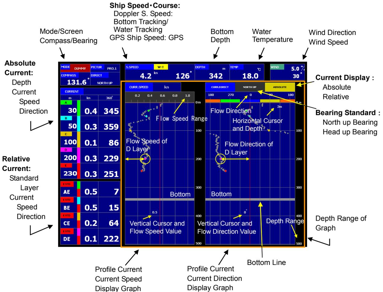
\*601 Depth in which the current can be measured is up to a depth value of about 80% of the bottom of the sea depth.
