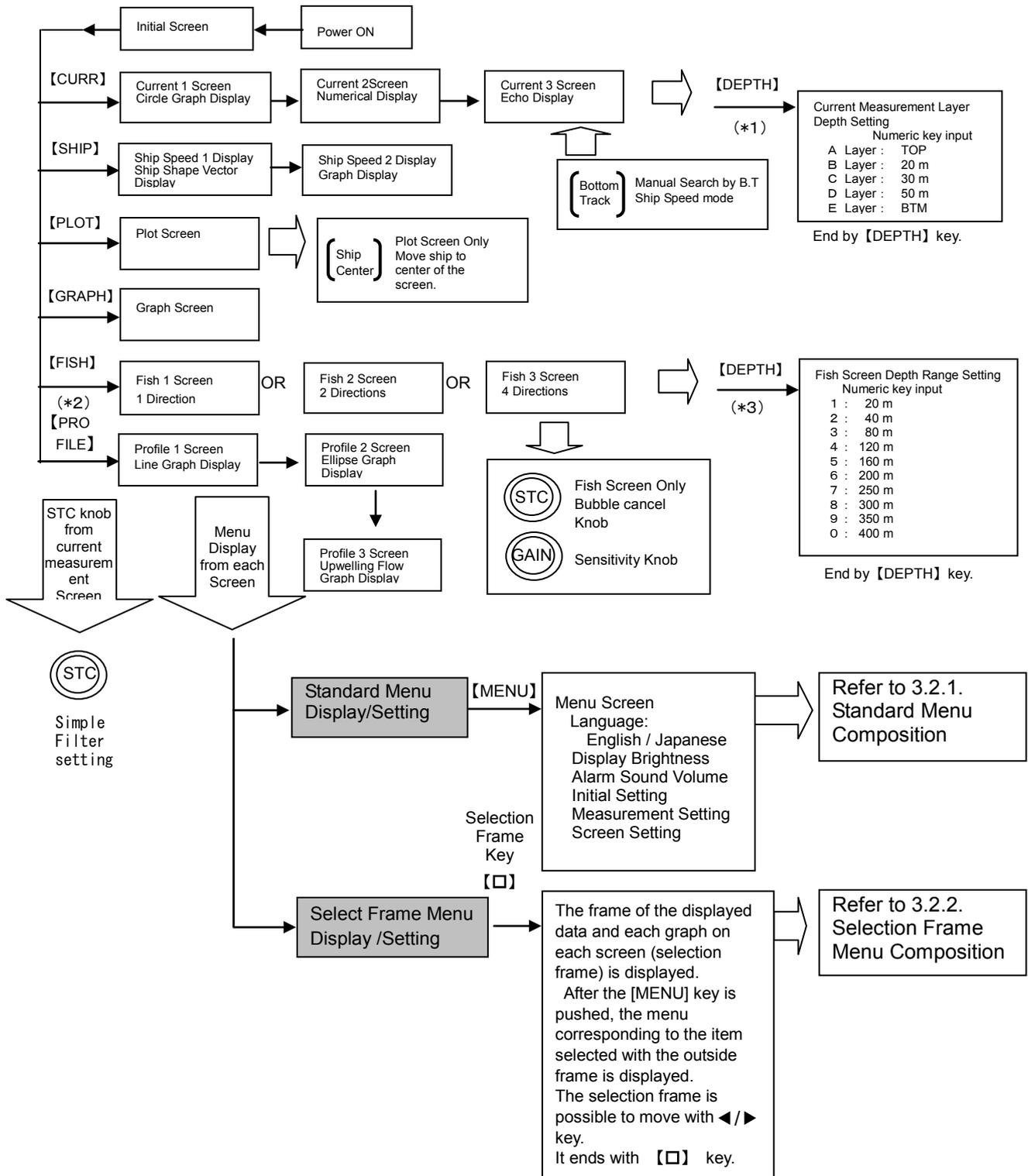
\*1 Depth setting in current measurement layer: Refer to 4.2.3 "Current Measurement Depth Setting"
