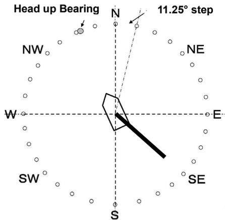
The graphical figure displays all surroundings with the bearing mark of division (11.25° step) into 32. (Figure 4.1.1)
