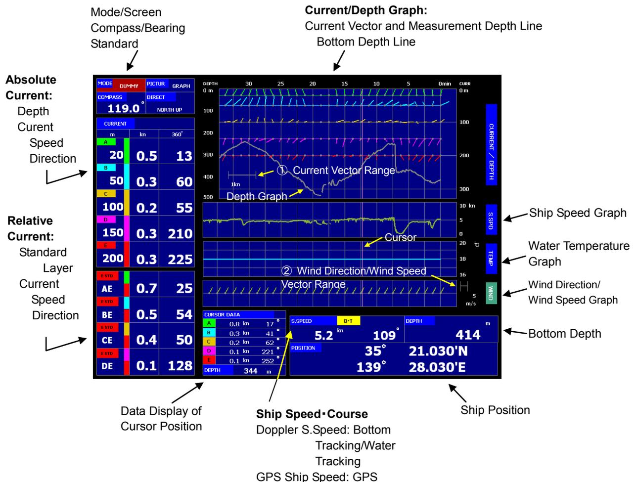
\*401 Water Temperature: It is necessary to connect the water temperature sensor for the display of the water temperature graph.
